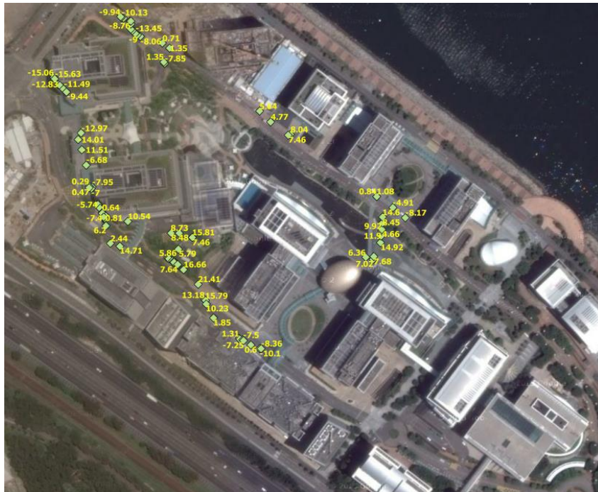
Figure 13: SINR measurement results (in dB) for Lakeside 2 base station.
