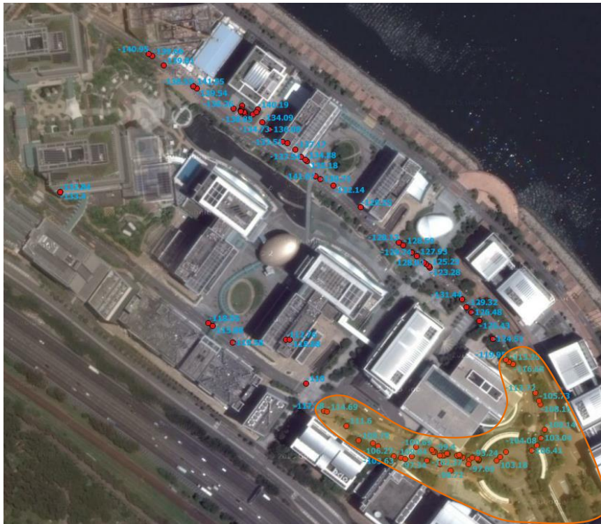
Figure 11: RSRP measurement results (in dBm) for Photronics Center base station.
