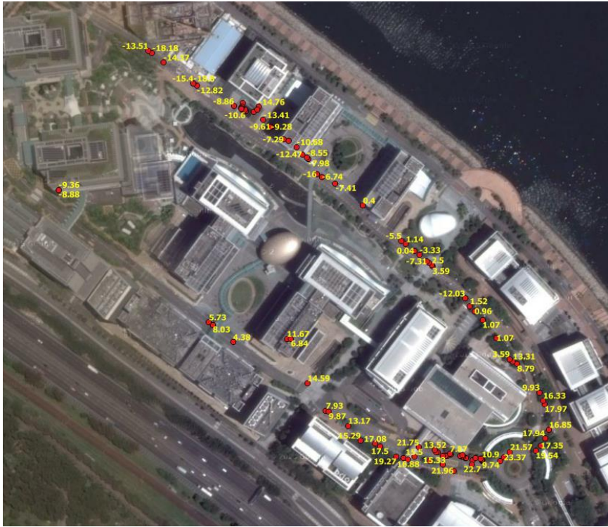
Figure 10: SINR measurement results (in dB) for Photronics Center base station.
