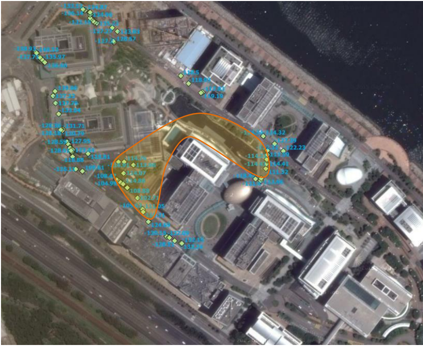
Figure 14: RSRP measurement results (in dBm) for Lakeside 2 base station.
