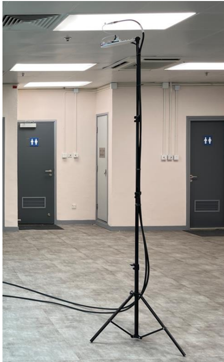
Figure 3: Setup of X-Pol omni antenna
